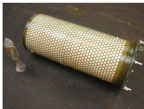
Fig. 12 A GRP + Derakane Resin Candle Filter
